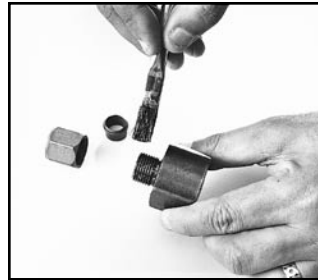
Step 1 – Lubricate thread and cone of Ferulset Tool (or fitting body).
